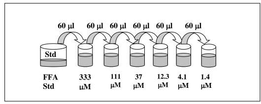
Note: The above dilution series generates enough volume to perform the standard curve in duplicate. If you wish to perform the standard curve in duplicate, please note that seven fewer data points can be assayed with this kit.
