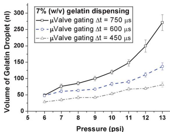
**Figure 3.** Mean droplet volume with standard error of 7% (w/v) gelatin solution ( $n=8$ ) with increasing pneumatic pressure to microvalve when the valve opening duration were 750, 600, and 450 μs. [Color figure can be seen in the online version of this article, available at [www.interscience.wiley.com](http://www.interscience.wiley.com).]
